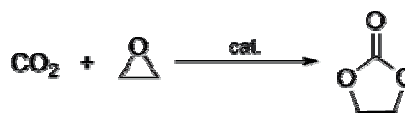
Figure 2. A simple example of an epoxide reacting with CO_2 in the presence of a catalyst.
