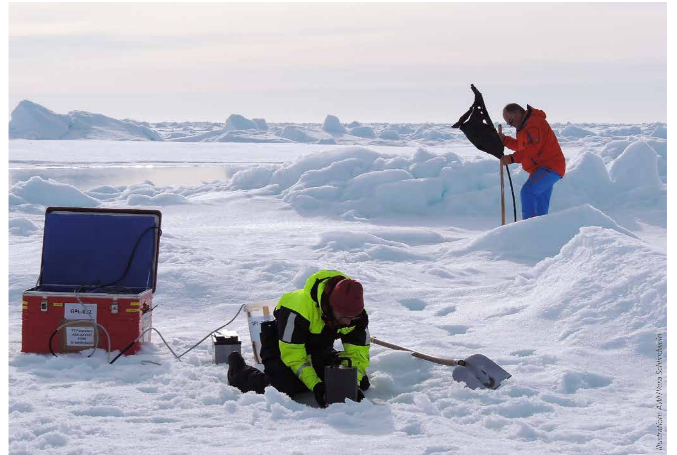
Hard at work in the icy cold: Setting up a seismometer on an ice floe in the Arctic sea ice.
