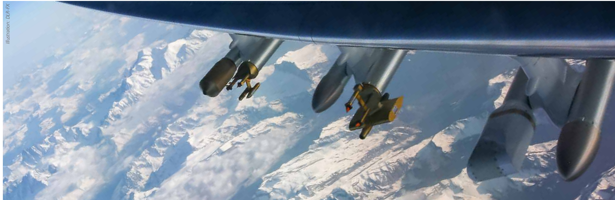
PMS (Particle Measurement System) probes can be mounted below HALO's wings. These systems allow high-precision in-situ measurements of aerosol particles, cloud droplets and ice crystals.
